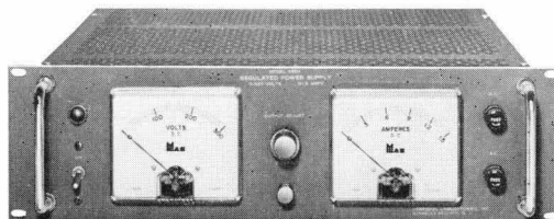
Fig. 10. High voltage (320 v) from an all solid-state supply is available in H-Lab's Model 895A, supplying up to 1.5 amps dc. "Piggy-back" regulator eliminates need for expensive high-voltage transistors.
